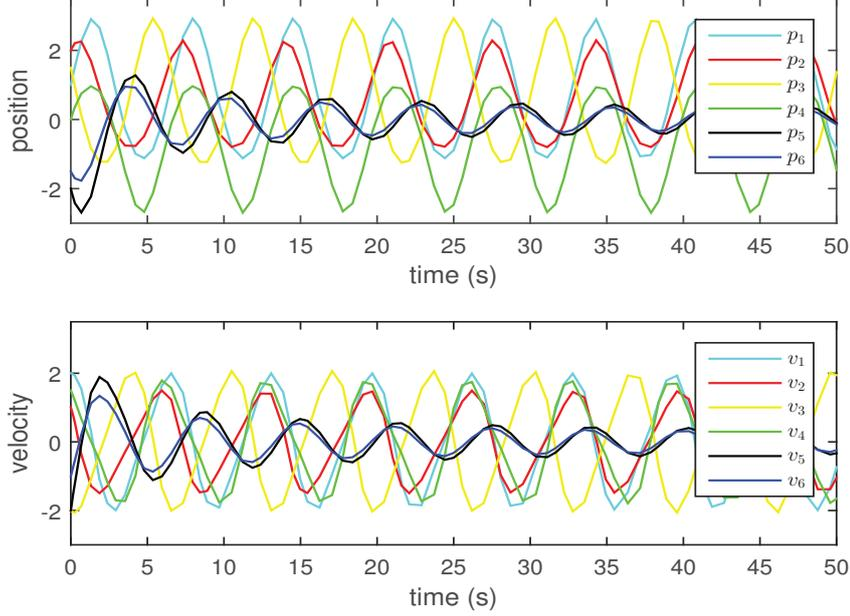
**Figure 5.2:** Profile of state trajectories of six agents without controller
