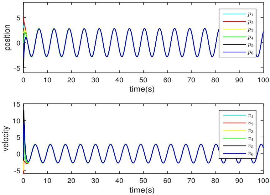
**Figure 4.5:** Profile of state trajectories of six agents with adaptive controller
