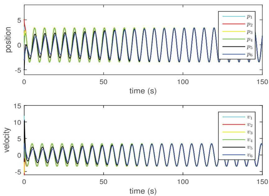
**Figure 4.8:** Profile of state trajectories of six agents with unknown constant parameters within interval  $[-50, 50]$
