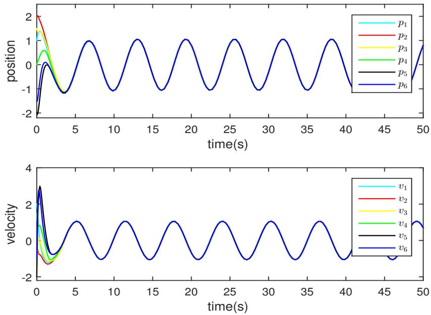
**Figure 5.5:** Profile of state trajectories of six agents with adaptive controller
