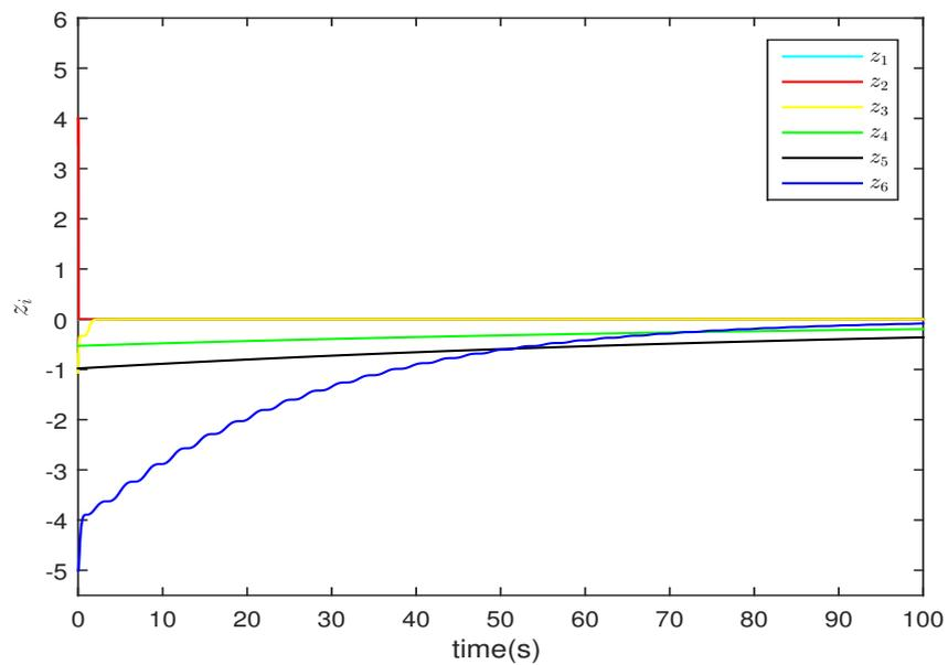
**Figure 4.7:** Profile of  $z_i$  of six agents with adaptive controller
