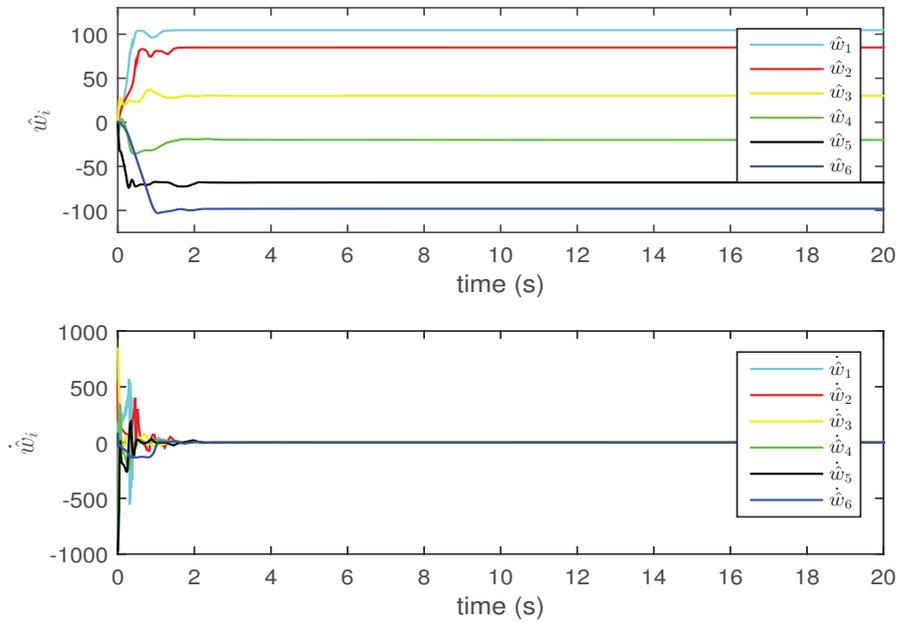
**Figure 3.9:** Profile of  $\hat{w}_i$  and  $\dot{\hat{w}}_i$  with adaptive controller and unknown constant parameters within interval  $[-100, 100]$
