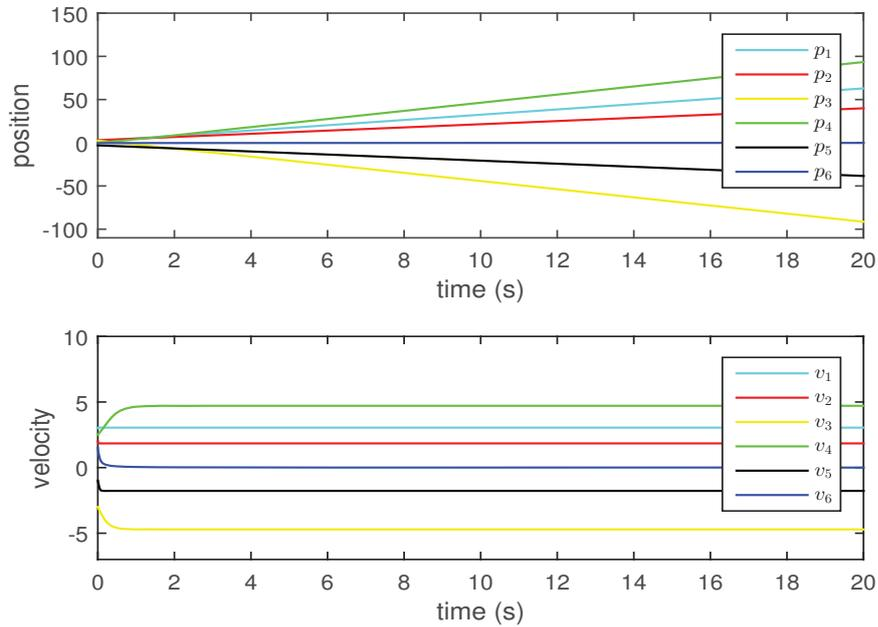
**Figure 3.2:** Profile of state trajectories of six agents without controller
