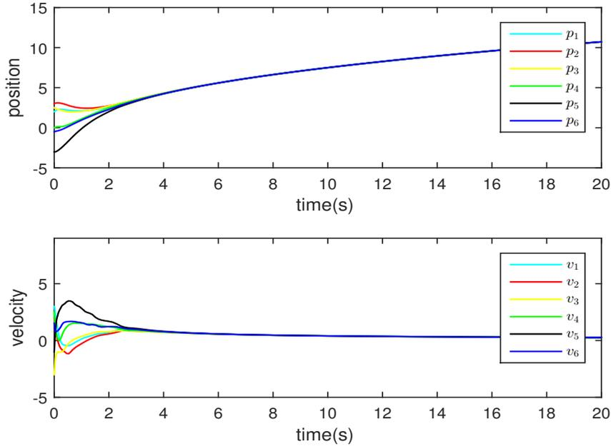
**Figure 3.5:** Profile of state trajectories of six agents with adaptive controller
